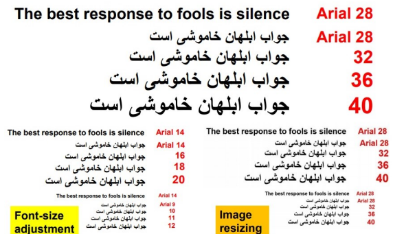
Fig. 17. Illustrating the quality of Persian script using the Arial font of different sizes (top) and the effects of font-size adjustment and image resizing on readability of the resulting text.
