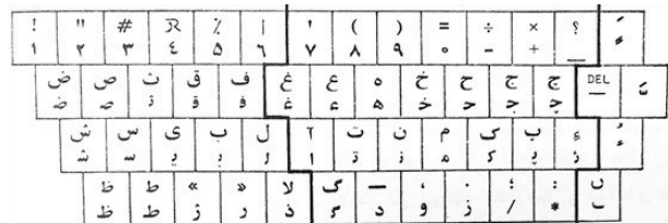
Fig. 11. Unified Persian keyboard layout, a proposed standard for computers, typewriters, and other data-entry systems [15].
