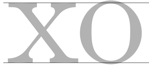
FIG. 7: The difference between the height of a glyph with a flat top segment and a glyph with a round top segment is called top overshoot . Analogously, the difference in depth is called bottom overshoot. Glyphs from the string ‘xzroesc’ are used compute the blue zone and overshoot value of the top and bottom of lowercase letters.
